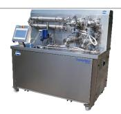
Best-In-Class Margarine Crystallizer Plug & Play High Pressure crystallizer, flexible configuration.
